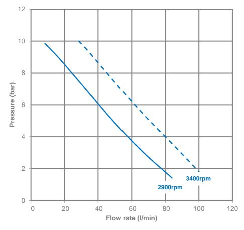
Above curves are valid for LPG with specific gravity of 0.56 kg/dm<sup>3</sup>
